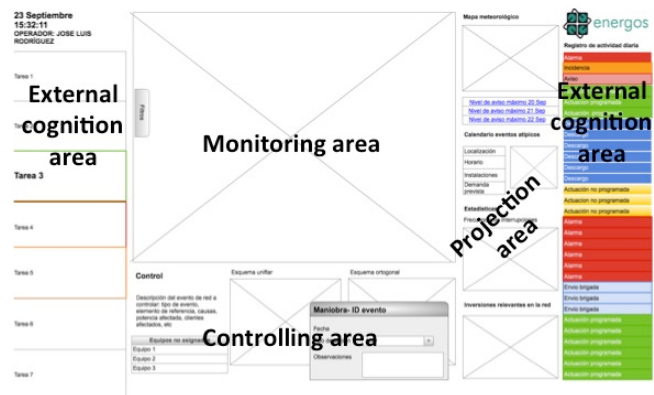
Figure 4. Low-fidelity prototype. The prototype was oriented to define the layout of the user interface
